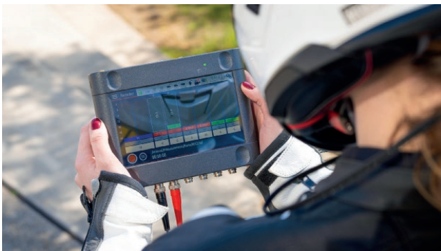
Motorcycle helmet connected to SQadriga III
