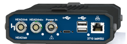
labHSU is a flexible binaural data acquisition system in the format of the HEADlab family
