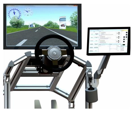
For convenient operation of H3S e.g. for switching between sound variants, a touch screen is attached via a pivoting arm on the operating console. During the simulation, H3S presents a visual driving simulation including current driving conditions such as RPM and speed via a monitor, which is centrally arranged behind the wheel.
