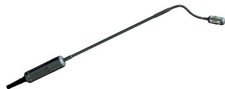
HEAD VISOR Probe (Code 7523) is used for acquiring low-frequency sound components with VMA V. HEAD VISOR Probe has two microphones in its tip which detect sound emitted by a surface of the measured object along with the exact sound location. The position of HEAD VISOR Probe itself is tracked and recorded by the VMA V cameras.
