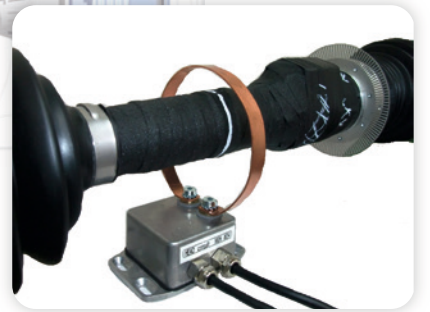
Torque and speed sensors on drive shaft
