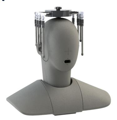
The microphone array MSA II mounted on an artificial head measurement system like HMS II.3 allows realistic recordings of individual background noise scenarios for testing ANC headphones and headsets.
