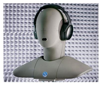
HEAD acoustics' testing solutions enable manufacturers to test and further develop state-of-the-art (ANC) headphones and headsets.
