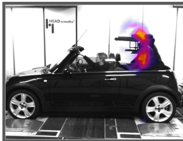
Figure 8: Sound source localization by means of beamforming
