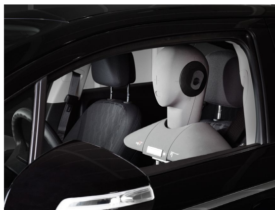
Example of a receiver sensor: Artificial head measurement system for performing BTPA
