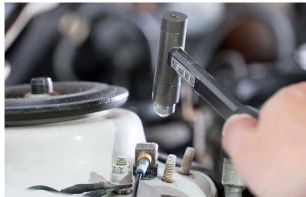
Determining the inertance by means of impact hammer measurements
