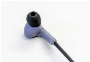
Fig. 1: Mock-up used to assess bone-conducted voice signal in the ear canal of human subjects
