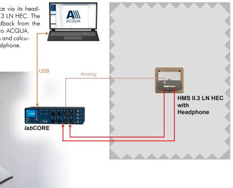
Configuration example 2: Measurement Setup for a Multichannel Loudspeaker System in a Vehicle
