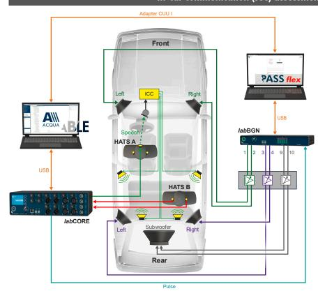
This example illustrates the assessment with ABLE of an in-car communication system. The assessment is executed with enabled as well as disabled ICC system for comparison.
