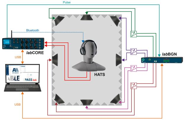
This example describes the assessment with ABLE of the active noise cancellation (ANC) performance from a headset including Bluetooth wireless technology. The assessment is carried out with ANC switched off and for comparison with ANC switched on.
