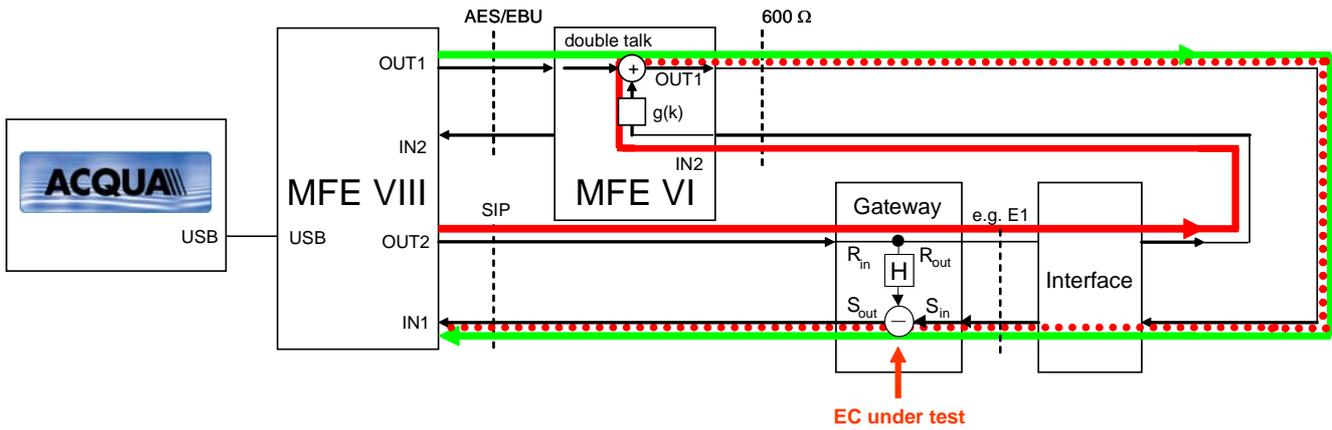
Configuration example for measurement of a gateway echo canceller with analysis system ACQUA and measurement front ends MFE VI and MFE VIII (green: sending direction, red: receiving direction). The echo path simulation  $g(k)$  and feeding of the double talk signal (DT) can be realized either by MFE VI or MFE VIII.
