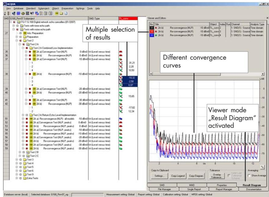
Example of Echo canceller tests with analysis system ACQUA. Several convergence measurements were carried out with the same SMD but with varying echo canceller settings. All resulting curves can be shown in one diagram using the multi-select features and the 'Result Diagram' tab of ACQUA
