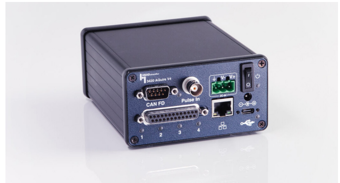
4-channel frontend AQuire V4
