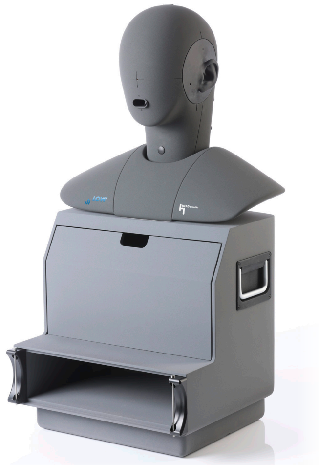
HMS II.3 ViBRIDGE mounted on the HTB VI torso box
