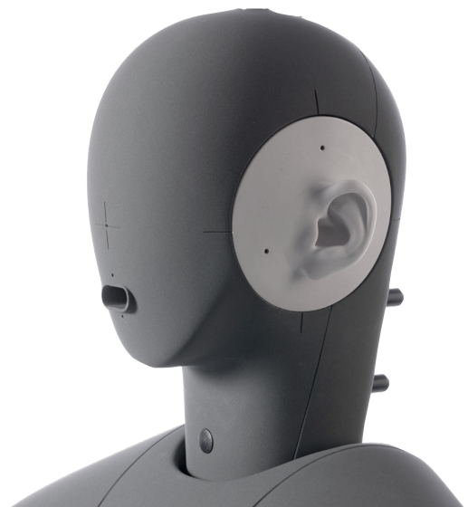
Type 4.4 pinnae are available in the colors dark gray and light gray. The light gray pinnae are available for retrofitting or initial delivery with HMS II.3 ViBRIDGE.
